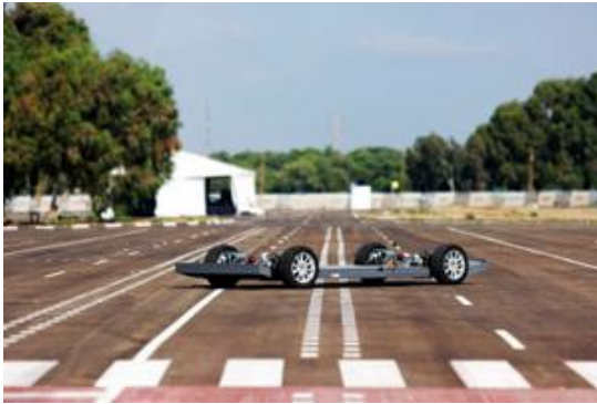
REE prototype platform for first phase of REEcorner™ and control technology validation tests for Navya's next-generation autonomous vehicles.
