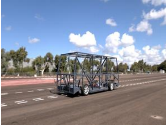
REE platform and frame that will be used to secure hardware such as lidars and sensors during completion of first phase of validation tests of REEcorner™ and control technology for Navya's next-generation autonomous vehicles.
